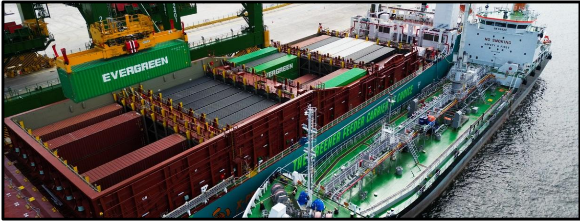
Ship to Ship Methanol Bunkering (Port Authority of Singapore)
