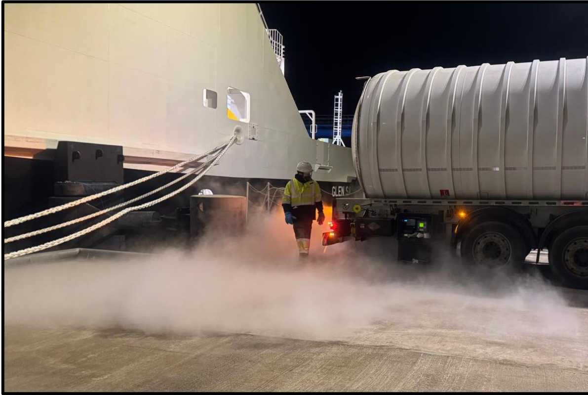
Truck to Ship LNG Bunkering (Waves Group)
